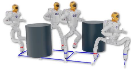
Fig. 4. R2 autonomously climbing handrails.
